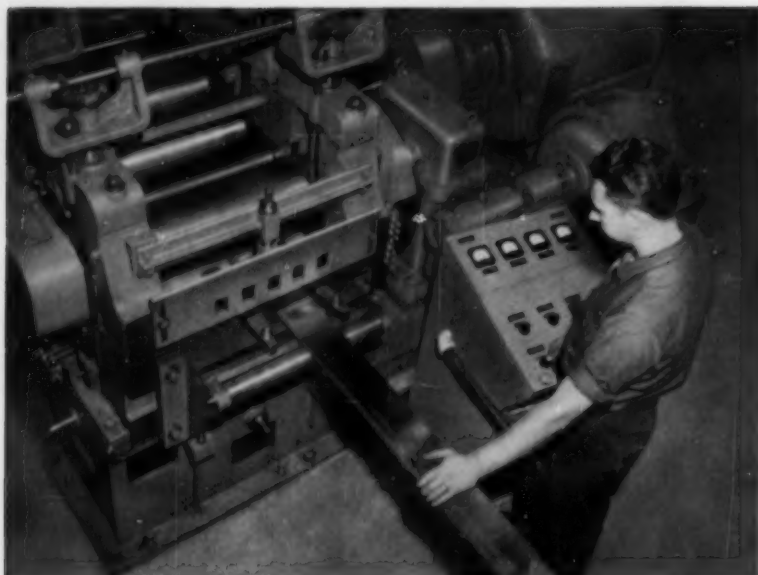
NEW ROTARY SCARFER shaves the outer surfaces of beryllium copper billets prior to hot rolling. Machine removes oxides, scale and dirt for a "pure roll."
